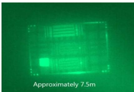
Figure 3: Image captured of test target with UTOFIA camera. Target can clearly be seen at 7.5 distance, 2.5 x longer than normal cameras.
