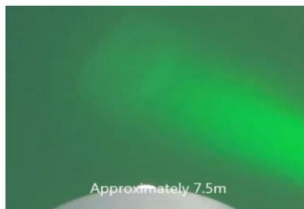
Figure 4: Image captured with GoPro camera for comparison. Target is almost invisible at 7.5 meter distance, where UTOFIA sees it clearly. At 3 meter distance, the target starts to appear for the GoPro camera.
