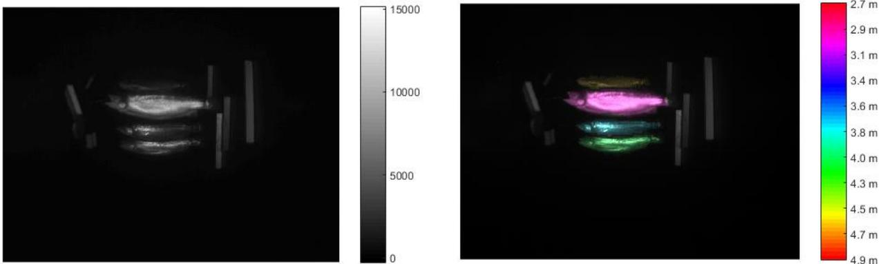
Figure 5: Regular image as usually acquired by cameras (left) and camera image with color-encoded depth information (right). In the top image it is difficult to ascertain the precise size of each fish, and which fish is behind which fish. By also directly measuring the distance to each fish, both precise size and relative fish position can easily be obtained.
