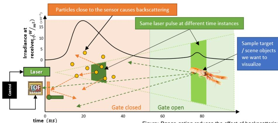
Figure: Range-gating reduces the effect of backscattering.
