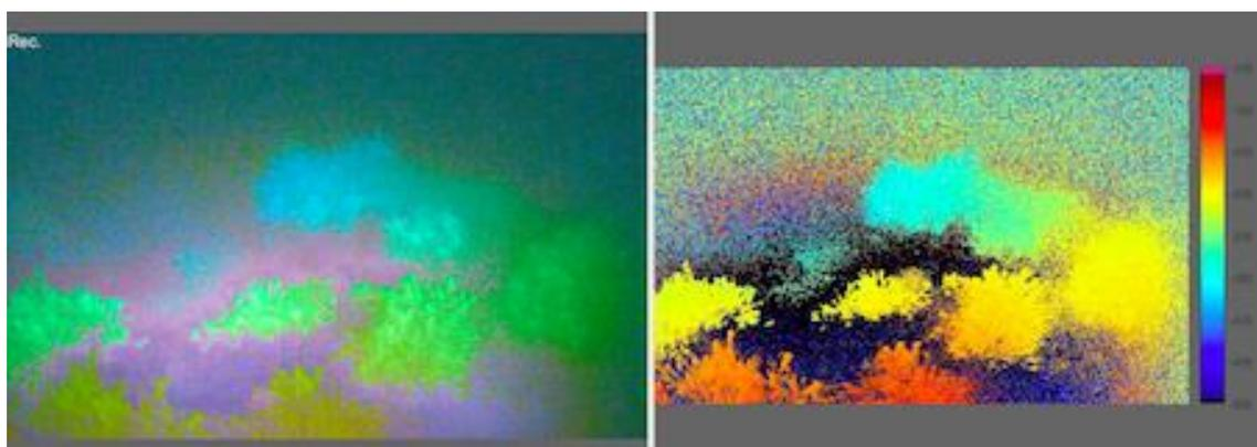
**Figure 2.** UTOFIA system 1 images for coastal substrate in Assens (Denmark) collected at 30 m depth. Left side shows the overlay functionality where the depth distance is over imposed on the camera image, while on the right side only the depth-distance is displayed with the associated colorbar.
