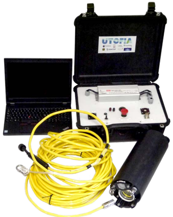
UTOFIA camera with supporting power box and cable
